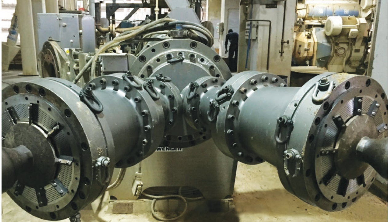
Wenger dual die head assembly for the AFX-3000 enables high volume output of extruded micro feed
