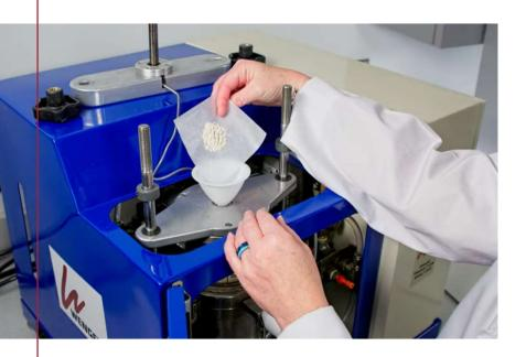
The PTA main unit consists of two sealed chambers, separated by an interchangeable capillary die, that prevents sample moisture loss so testing can be at temperatures far exceeding 100°C.
